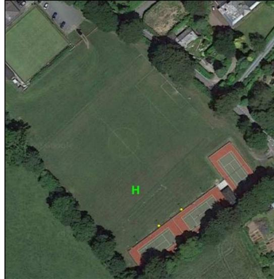
Photo: Shows the community landing site at Yelverton Recreation Field; the yellow dots indicate the two new floodlights (secured to the existing columns by the tennis courts) and 'H' the area used for night operations (N.B. no markings are required at the night landing site).
